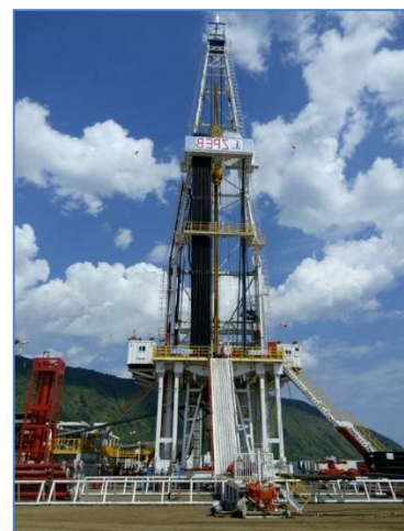
Photograph 2-1: A drilling rig at Lake Albert, about 45 m high
