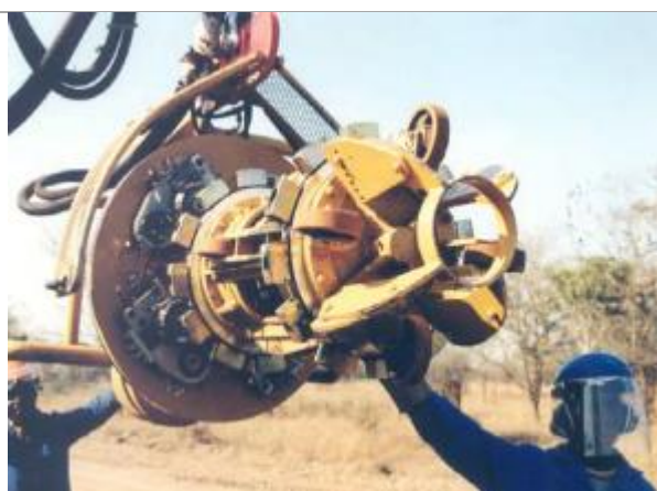
Bevelling machine for trimming pipe ends
