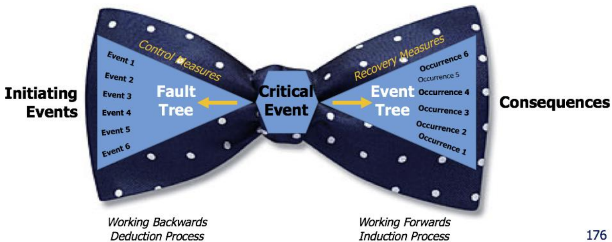
Figure 10-10: The principles of a bow-tie (Source: University of Toronto / Minerva, 2015, Rev. 4)
