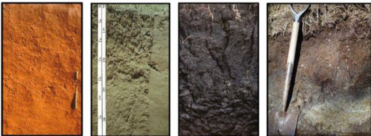
Figure 6-15: Examples of FAO classified soils (from left to right) - Ferrasols, Lithosols, Vertisols and Gleysols
