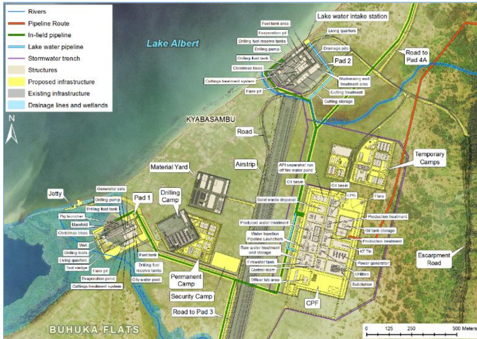
Figure 2-21: Footprint and typical layout of the CPF, showing the context of the well pads and associated infrastructure
