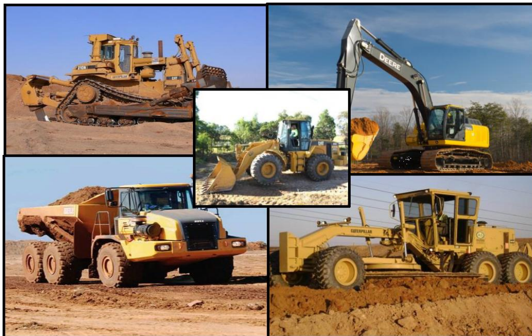
Figure 25: Dozer, excavator, tipper, grader and front end loader earth moving equipment.
