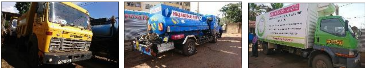
Figure 5: Examples of Modified Dump Truck (left), Vacuum Tanker (centre) and Box-body Truck (right)
