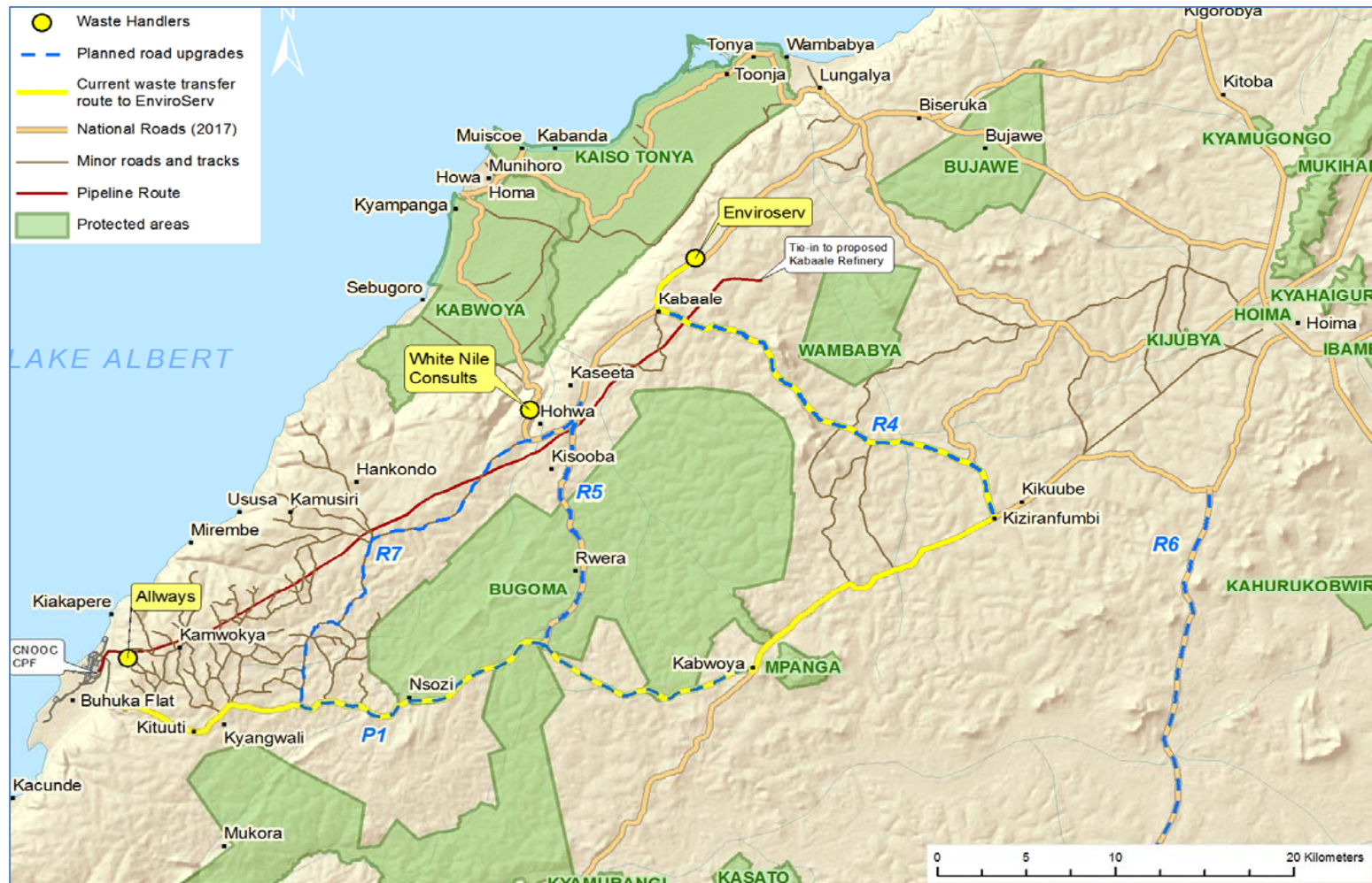
Figure 39: Regional road upgrades proposed above the escarpment
